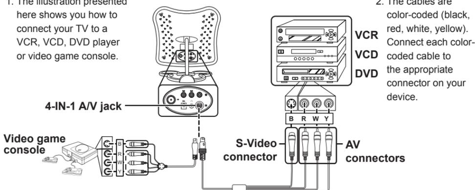
2. The cables are color-coded (black, red, white, yellow). Connect each color-coded cable to the appropriate connector on your device.
