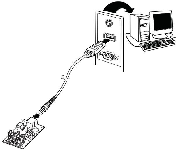
If using high-speed USB, connect the USB interface cable to side of the engine and to the USB port on the computer.
