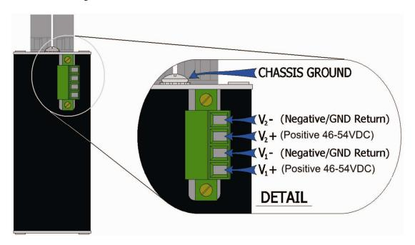
Unscrew & Remove the DC Voltage Input Plug from the top header.
