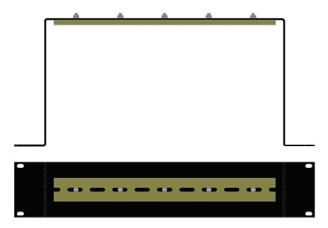
Most N-Tron<sup>TM</sup> products designed to be mounted on industry standard 35mm DIN rail. However, DIN rail mounting may not be suitable for all applications. Our Rack Mount Assembly (P/N: 900-RM) may be used mount to the 105TX/FX-POE enclosures to standard 19" racks as an option.
