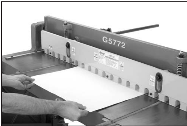
Figure 28. Example of a paper shear test.
