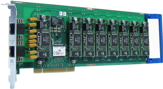
The MultiModem® ISI server card is ideal for small- to mid-sized companies requiring analog dial-up remote access or a dedicated fax server solution. It provides up to eight built-in V.92/56K modems for cost-effective, high-density, server-based remote access. The MultiModem ISI server card also offers V.34/33.6K Super G3 fax and Error Correction Mode, that can reduce fax transmission time by more than half when compared to traditional fax modems.
