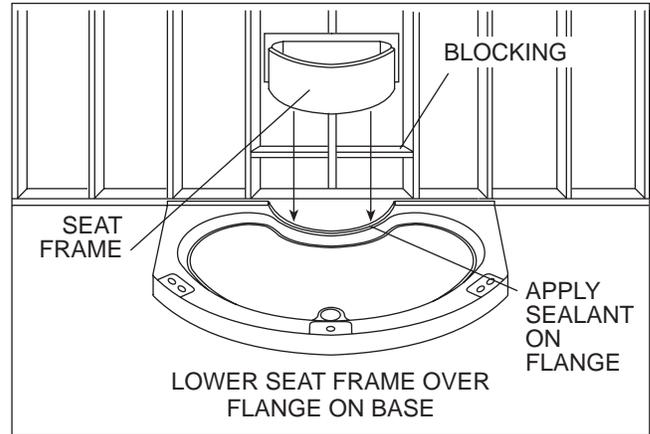
**NOTE:** If there is any gap between seat frame flange and stud or blocking, shims **MUST** be used to prevent distortion or cracking of the flange. See Shim Instructions.
