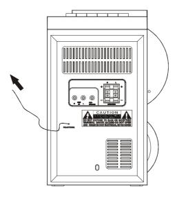
**AM**: The AM bar antenna is inside the cabinet of the main unit. You may need to change the position of the main unit until you find the position that provides the best reception for your favorite AM stations.
