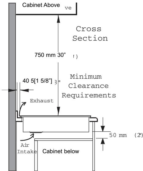
A minimum vertical clearance of 750 mm [30"] is required between the top of the cooking surface and the bottom of any unprotected combustible material, such as cabinets, wooden trim etc.
