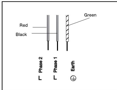
responsible for any unit malfunction due to an inadequate electrical supply (inadequate cable size, low voltage, power surge etc). Furthermore, if your residence has only a 208 V supply system, and if the voltage frequently fluctuates, your cooktop may not function properly
