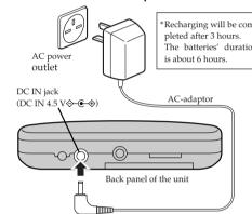
cannot be used to charge rechargeable batteries other than those AC adaptor from the power outlet and the optional car adaptor as required. DC IN jack
