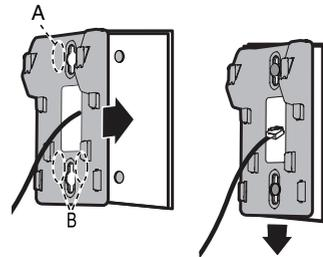
3. Align and place the telephone base on the wall mount bracket. Slide it down until it clicks securely in place.
