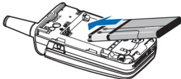
1. Insert the battery, gold-coloured contact end first, into the battery slot.
