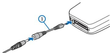
1. Plug the charger transformer into a standard ac outlet.
