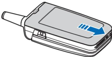
1. With the back of the phone facing you, press down and hold the back cover latch.
