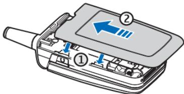
1. Set the back cover on the phone with the cover tabs aligned with the slots in the phone.
