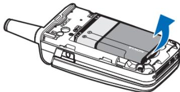
After you have removed the back cover, insert your finger into the finger grip, and lift the battery from its compartment.
