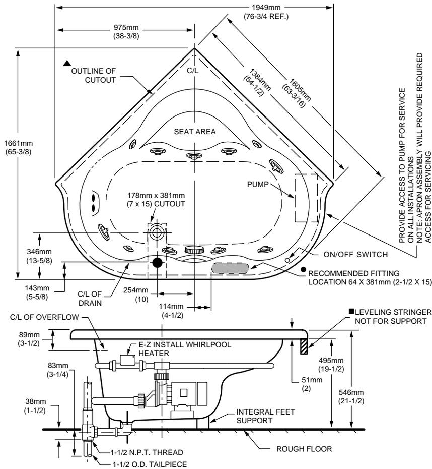
PROVIDE ACCESS TO PUMP FOR SERVICE ON ALL INSTALLATIONS. NOTE: APRON ASSEMBLY WILL PROVIDE REQUIRED ACCESS FOR SERVICING
