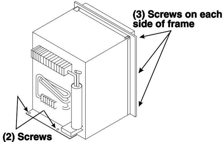
**NOTE:** Push refrigerator into enclosure until front frame is tight against the cabinet. First, secure the frame to cabinet with six screws. Second, install the two screws to the floor at the rear of the refrigerator.
