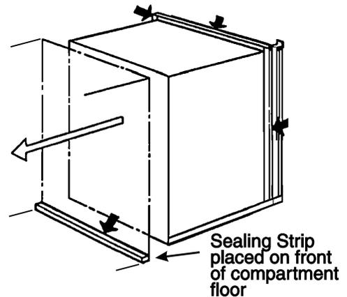
**NOTE:** Be careful not to damage the sealing strip applied to the floor of the enclosure when the refrigerator is put in place.
