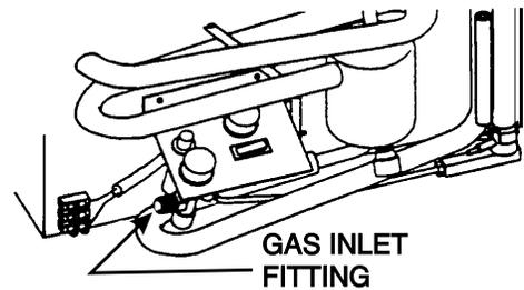
The gas supply system must incorporate a pressure regulator to maintain a supply pressure of not more than 13.5 inches water column, static (no load).
