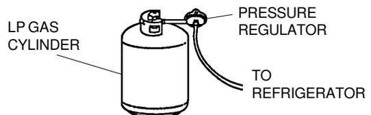
When testing the gas supply system at test pressures in excess of 1/2 psig, the refrigerator and its individual shutoff valve must be disconnected from the gas supply piping system.
