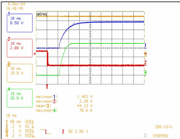
Start-up from on/off Switch, 48Vin, Full Load, Cext,min.
