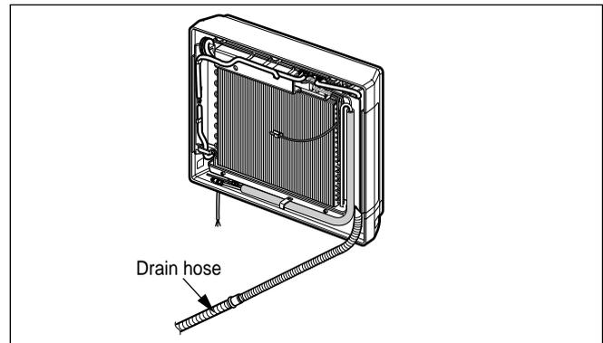
2. Tape the tubing, drain hose and the connecting cable. Be sure that the drain hose is located at the lowest side of the bundle. Locating at the upper side can cause drain pan to overflow inside the unit.
