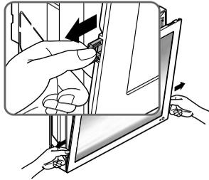
3. Push and close the top part of the front panel and then pull the bottom part of the panel forward until it is secured.
