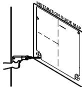
5. Drive the fore plastic anchors into drilled points.
