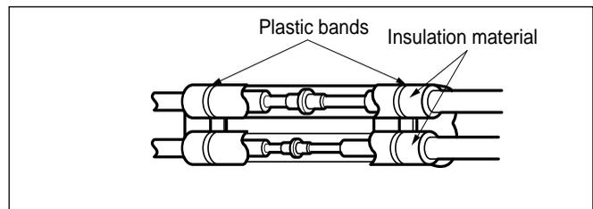
3. Bundle the piping and drain hose together by wrapping them with vinyl tape over the range within which they fit into the rear piping housing section.
