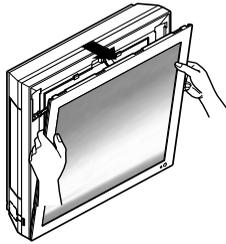
2. Pull out the both links of lower part of front panel, as described in the below picture.
