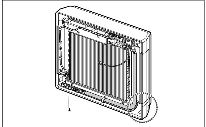
2. Assemble connecting lead wire with controller, fix the upper part of panel front, and match the lower part of panel front.
