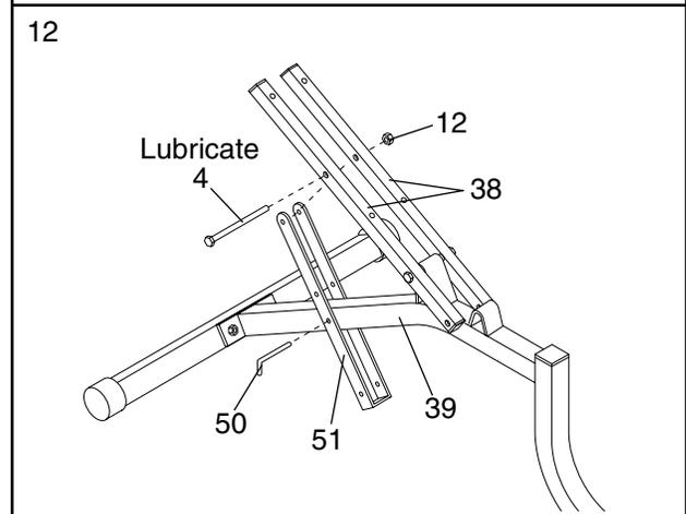
13. Lubricate an M10 x 127mm Bolt (4). Attach the Seat Frame (44) to the Backrest Brackets (38) with the M10 x 127mm Bolt and an M10 Nylon Locknut (12). **Do not overtighten the Nylon Locknut; the Backrest Brackets and Seat Frame must be able to move freely.**
