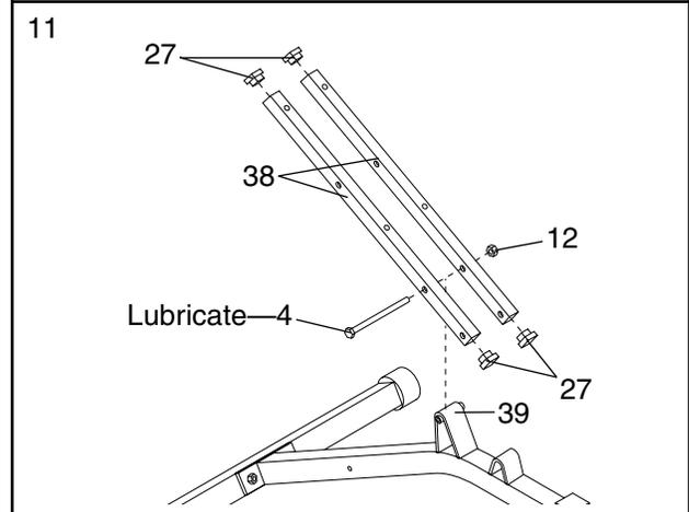
12. Lubricate an M10 x 127mm Bolt (4). Attach the Adjustment Bracket (51) to the Backrest Brackets (38) with the M10 x 127mm Bolt and an M10 Nylon Locknut (12). **Do not overtighten the Nylon Locknut; the Backrest Brackets and Adjustment Bracket must be able to move freely.**
