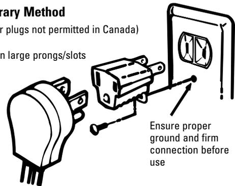
**CAUTION:** Attaching the adapter ground terminal to the wall receptacle cover screw does not ground the appliance unless the cover screw is metal, and not insulated, and the wall receptacle is grounded through the house wiring. The customer should have the circuit checked by a qualified electrician to make sure the receptacle is properly grounded.
