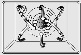
In a convection oven, a fan circulates hot air over, under and around the food. This circulating hot air is evenly distributed throughout the oven cavity. As a result, foods are evenly cooked and browned—often in less time than with regular heat.
