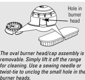
The oval burner head/cap assembly is removable. Simply lift it off the range for cleaning. Use a sewing needle or twist-tie to unclog the small hole in the burner heads.
