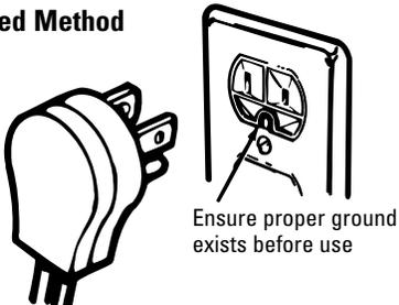
The power cord of this appliance is equipped with a three-prong (grounding) plug which mates with a standard three-prong grounding wall receptacle to minimize the possibility of electric shock hazard from this appliance.
