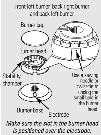
Make sure the slot in the burner head is positioned over the electrode.
