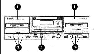
**4** Press the NORMAL DUBBING button for normalspeed copying or the HIGH DUBBING button for high-speed copying, and the taping starts.
