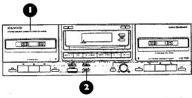
3 Set the Dolby Noise Reduction mode by moving the switch to the proper setting for the tape you're playing. For example, if your playing a tape recorded using Dolby C, select Dolby C.
