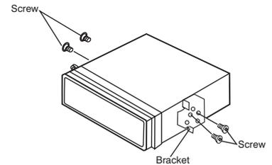
Installation using the screw holes on the sides of the unit. Fastening the unit to the factory radio mounting bracket.
