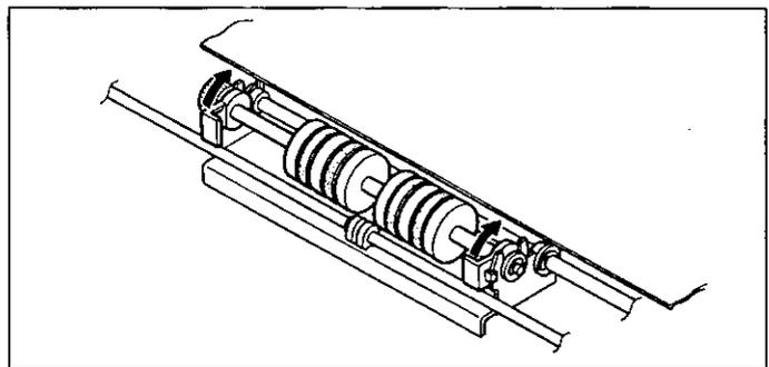
**4** While pushing down the metal holder of the retard roller module, remove the retard roller module.
