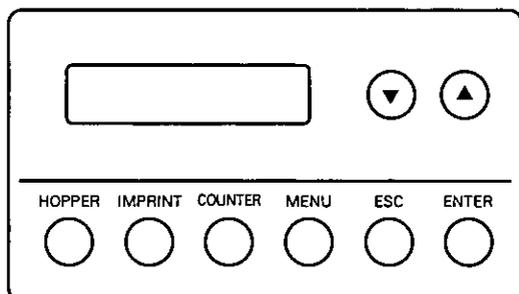
**HOPPER** : Press when changing the hopper position to the next position.
