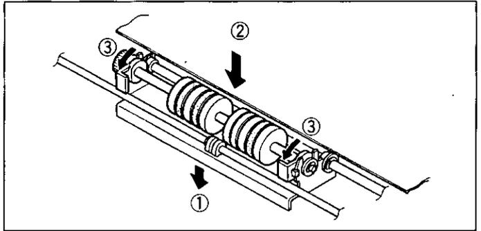
**7** Hold the paper feed cover using both hands, install it in the scanner when installing the paper feed cover, the two hooks must securely latch on the scanner pins. Check that the hooks are securely latched by viewing through the small openings A. Push it into place until you hear a clicking sound.
