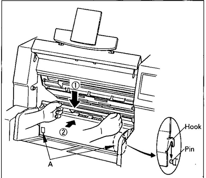
**8** Install the paper feed roller module which was removed in step 1, and close the front door which was opened.
