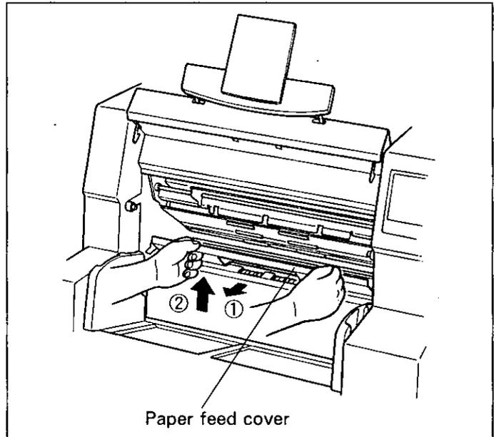
**3** Use your fingers to push up the two levers at both ends of the retard roller module.
