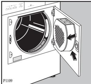
If necessary the filters can be cleaned under running water using a brush. In this case remove the filter in the door opening as per picture (it can be positioned with the tooth facing to the left or to the right).
