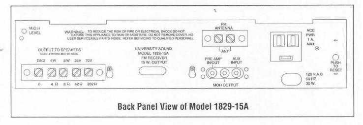
When using a MOH system with an 8 Ohm input, do not connect the input to the 8 Ohm output of the receiver, as it will overload the MOH circuit. Instead connect the 8 Ohm winding of a 25/70.7 Volt line matching transformer tapped in the area of 1/4 to 1/2 Watt.
