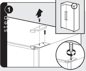
Remove and discard screw and hinge cover, if applicable. (Repeat if two hinges are used.)
