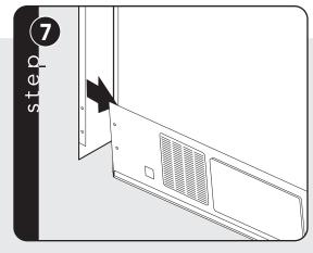
Attach rear of side panels with screws.
