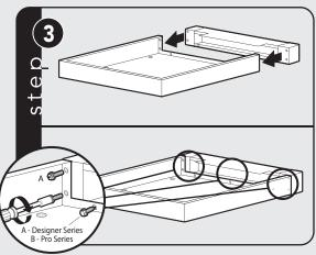
With top panel and grille upside down, position grille assembly in front of top panel. Secure top panel to grille assembly via four outer holes and three inner holes.
