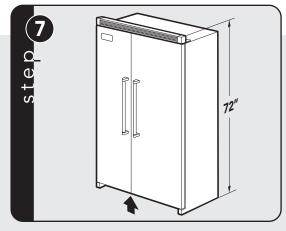
Raise the unit up until the measurement from the floor to the top of the grille assembly is 72 inches or 6 feet.
