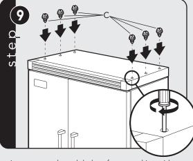
Insert screws through holes of top panel into side
