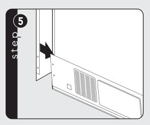
Attach rear of side panels with screws.
