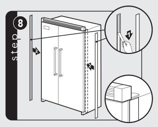
Shim trim has adhesive backing on both sides. Remove adhesive backing on refrigerator side only. Fit the shim trim to the front of the unit first. Locate the top of the shim trim with the top of the refrigerator cabinet.
