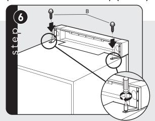
Secure the grille brackets to the holes in the hinge plate with two B screws.
