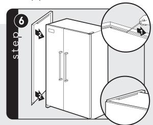
Remove adhesive backing from other side panel. Fit the side panel to the front of the unit first. Spacer on top of side panel needs to sit on top of refrigerator cabinet.
