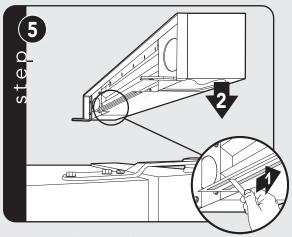
Remove adhesive backing. Firmly press the grille assembly down so the adhesive adheres to the cabinet.
