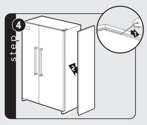
Remove adhesive backing from the side panel. Fit the side panel to the front of the unit first.
