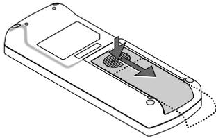
**2** Install new batteries (AAA). Ensure that you have the batteries' polarity (+/-) aligned correctly.
