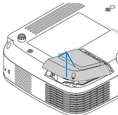
3. Loosen the two screws securing the lamp housing until the phillips screwdriver goes into a freewheeling condition. The two screws are not removable. Remove the lamp housing by holding it.
