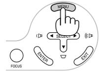
2. Press the **SELECT** ▲▼ buttons on the remote control or the projector cabinet to highlight the menu for the item you want to adjust or set.
