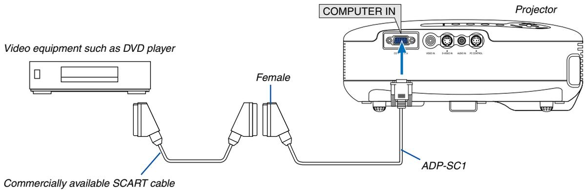
Before connections: An exclusive SCART adapter (ADP-SC1) and a commercially available SCART cable are required for this connection.
