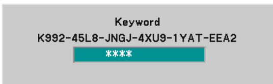
**Type in the correct keyword and press the ENTER button. The projector will display an image.**
