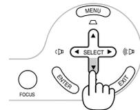
3. Press the **ENTER** button on the remote control or the projector cabinet to select a submenu or item.
