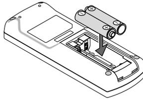
**3** Slip the cover back over the batteries until it snaps into place. Do not mix different types of batteries or new and old batteries.
