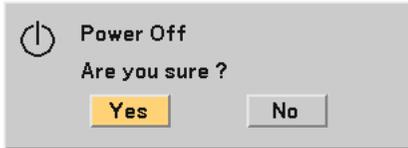
Secondly, press the **ENTER** button or press the **POWER (ON/STAND BY)** or the **POWER OFF** button again.
