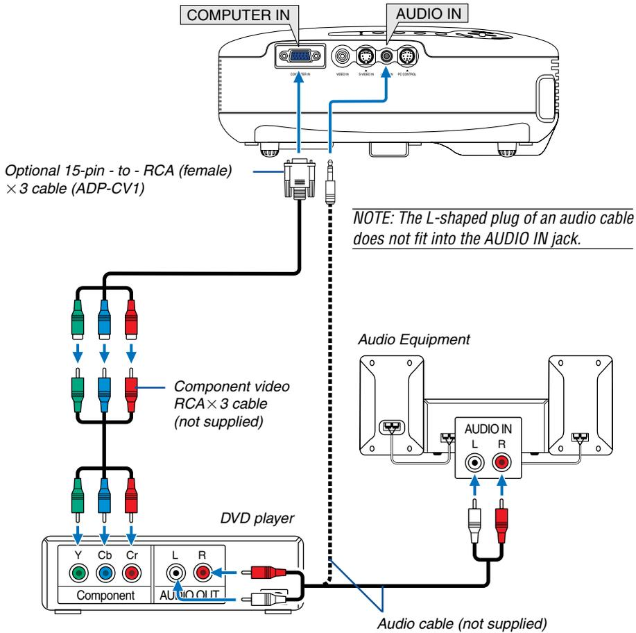
A component signal will be automatically displayed. If not, from the menu, select [Setup - Options] → [Signal Select] → [Computer], and then place a check mark in the “RGB/Component” radio button.
