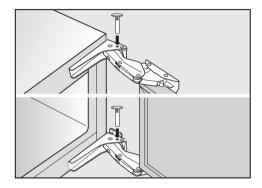
Place the locking pins supplied for limiting the door opening into the hinges from above.
