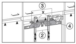
Undo nuts 3 and take fixing bracket4 off together with fitting aids 2.
