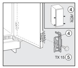
Screw fixing bracket ④ using hex screw ⑤ to the pre-drilled holes in the appliance door.
