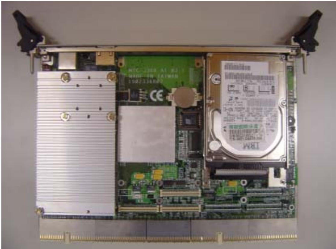
**Figure 1-5:** Complete assembly with heat sink and hard disk
