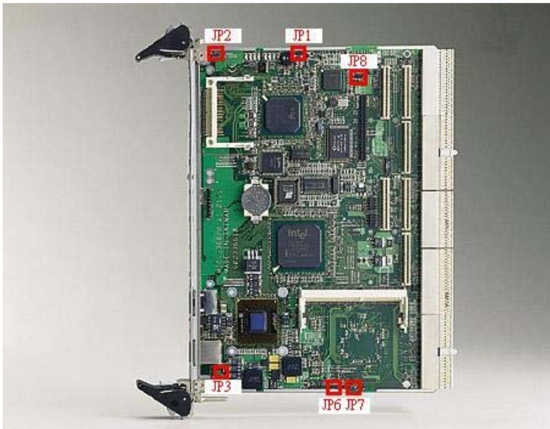
**Figure 1-2:** MIC-3368 jumper and connector locations.
