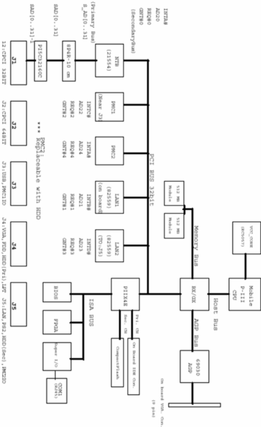
Figure 1-1: MIC-3368 functional block diagram.
