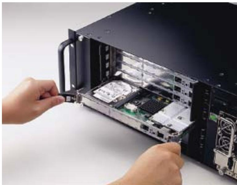
**Figure 2-1:** Installing the card into the chassis
