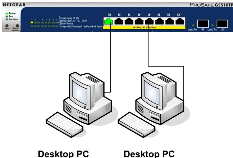
**Figure 5. Connect PCs to the Switch's RJ-45 Ports**
