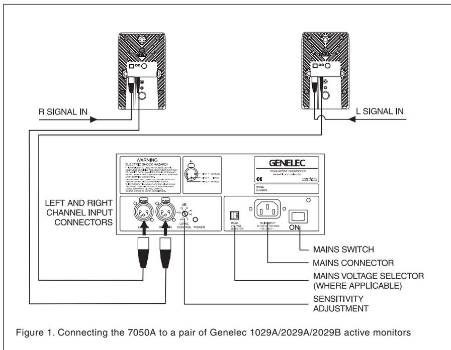
Figure 1. Connecting the 7050A to a pair of Genelec 1029A/2029A/2029B active monitors
