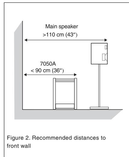
Figure 2. Recommended distances to front wall
