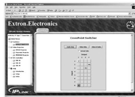
Example of screen to control an Extron CrossPoint matrix switcher.
