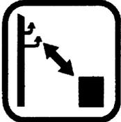
This unit is not designed to insulate against hazards associated with the contact of wires carrying electrical current. To avoid possible injury/death due to electrical shock or other hazards. **DO NOT** operate unit if any wires (power, telephone, cable, etc.) are closer than 15 feet (4/5 meters minimum distance, to any part of the unit or operator.
