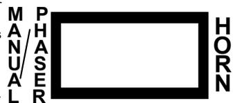
**Phaser** - With selector switch in **Wail** or **Yelp**, this tone override is toggled on and off by repeatedly pressing switch. A very rapid changing tone used at intersections and very highly congested areas. May be optionally replaced with **Two-Tone** or disabled. Two-Tone is two alternating frequencies like a European. See OPTION SWITCHES section.
