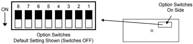
**SW-1 Auxiliary Input Polarity** - The auxiliary input is normally activated with positive, turn this switch ON for negative activation.
