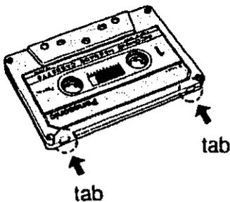
The tape can be erased even if the record-prevention (knock-out) tabs have been removed.
