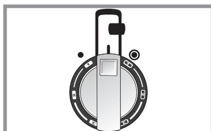
**5** The drawing by each knob indicates which area that knob controls. This one is the right hand dual circuit control. The setting you need depends on the kind of pan you use and the quantity of food. Higher settings are required for larger quantities of food.
