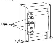
The primary taps (on one side of the transformer) are the inputs and are rated in watts. The secondary taps (on the opposite side of the transformer) are the outputs and are rated in ohms.
