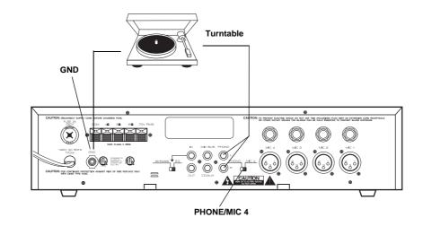
You can connect a low-level audio input source (such as a magnetic cartridge turntable) to the **L PHONO** and **R PHONO** jacks on the back of the amplifier.
