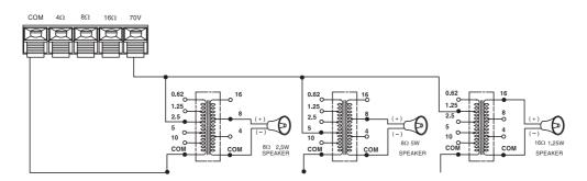
Connect a wire from **70V RMS** on the back of the amplifier to the transformer's desired primary tap (10, 5, 2.5, 1.25 or 0.62 watts).
