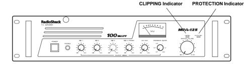
The CLIPPING indicator lights when a sound source's signal exceeds its mixing control setting. If this happens, reduce the level of the appropriate mixing control or reduce **MASTER VOLUME** until the indicator flickers only at peak volume levels.
