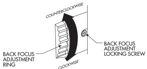
Figure 5. Back Focus Adjustment
