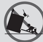
**WARNING:** To reduce risk of tipping of the appliance from abnormal usage or by excessive loading of the oven door, the appliance must be secured by a properly installed anti-tip device.
