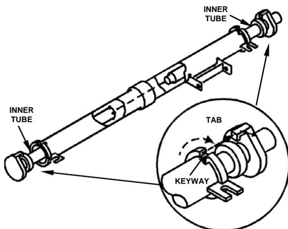
**Water Distribution Tube Disassembly**
