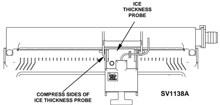
**Ice Thickness Probe Removal**
