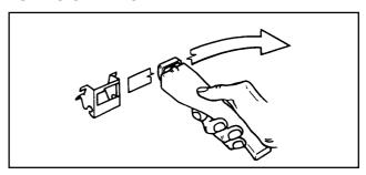
To correctly locate the grill pan on the shelf, ensure that the cut out on the underside of the handle bracket locates over the front bar of the shelf.
