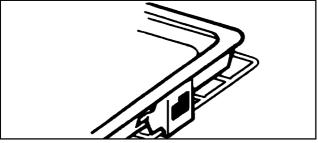
To check the progress of the food being grilled, the grill pan should be withdrawn on the shelf to attend to food during cooking or the carrier shelf can be lifted away from the cooker and rested on a heat resistant work surface.
