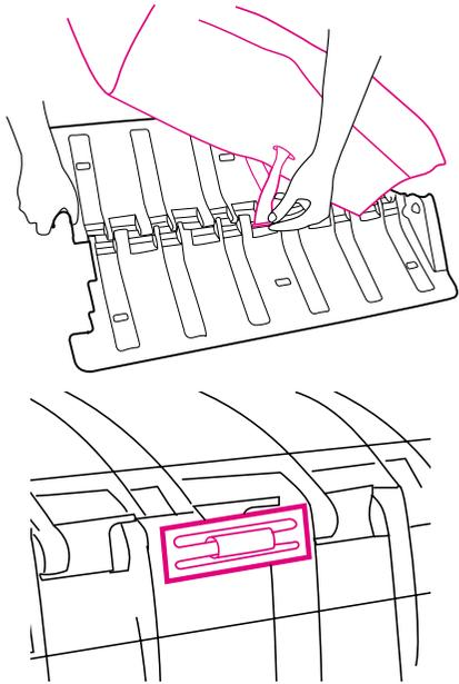
**⚠WARNING** Avoid falls. The waist belt must be secured by placing the plastic retainer through the opening between the two parts of the changing table. Check that retainer lays flat on the back of the changing table.
