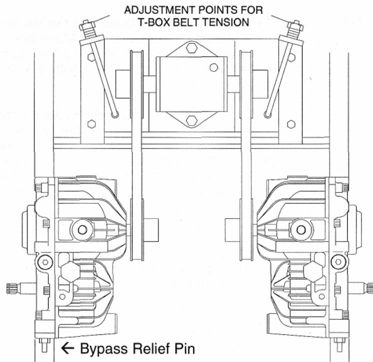
Each hydrostat has a bypass relief pin located at the rear of the hydrostatic unit. A bypass keeper is provided to allow the mower to be rolled around without complete servicing of the unit. To accomplish this, the bypass keeper springs must be positioned to depress the bypass relief pins. Remove bypass keeper springs prior to actual operation of the mower.
