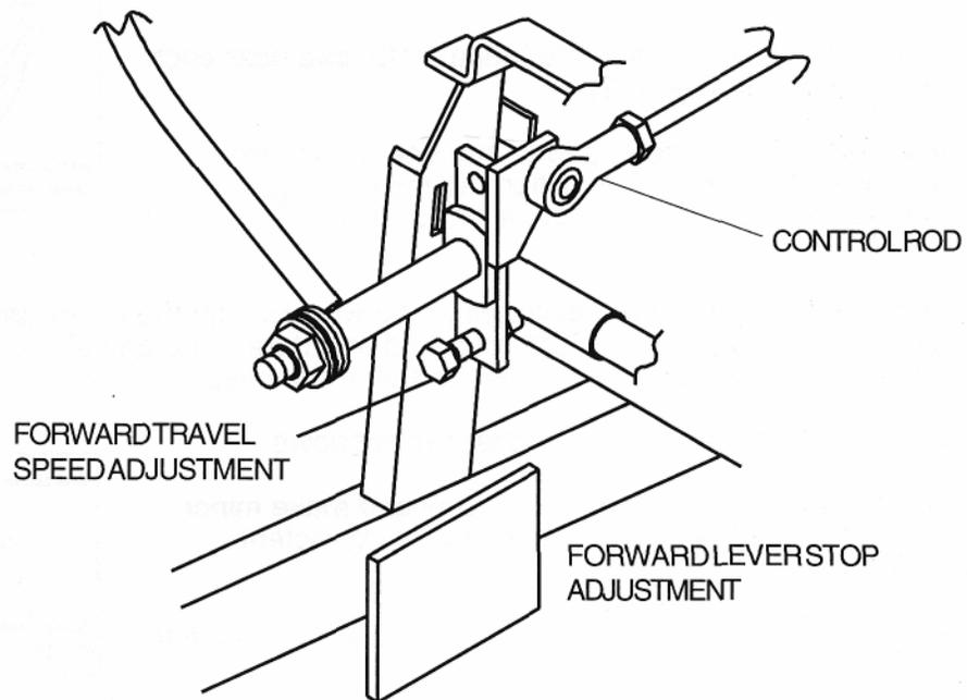
**NOTE:** Balance of travel speed. If mower tends to pull to either side, re-adjust lever stop on fast side to slow the hydrostat down and even out the ground speed.
