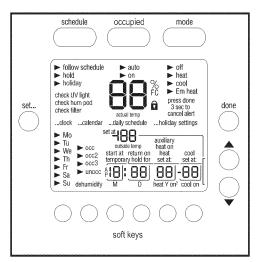
Fig. 2 — Thermostat Front Panel Buttons
