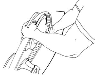
2. Rotate the L-wrench counter-clockwise to tighten the sheaves while working the belt to the outer edge of the sheaves.
