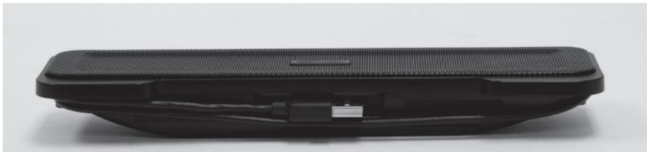
**Step 2** - On the back of the Portable USB Soundbar, rotate stand to the down position.
