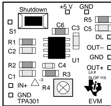
Figure 3–3. TPA301 EVM Schematic Diagram
