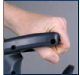
2. To stop the Hedge Trimmer move the Hedge Trimmer away from the cutting area and release either one of the switches.
