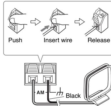
Once your T-4355 is ready for use, you'll need to tune into an AM radio station and adjust the position of the AM antenna to achieve the best possible reception.
