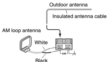
Outdoor AM antennas work best when installed outside horizontally, but good results can sometimes be obtained indoors by mounting horizontally above a window. Note that the AM loop antenna should be left connected.
