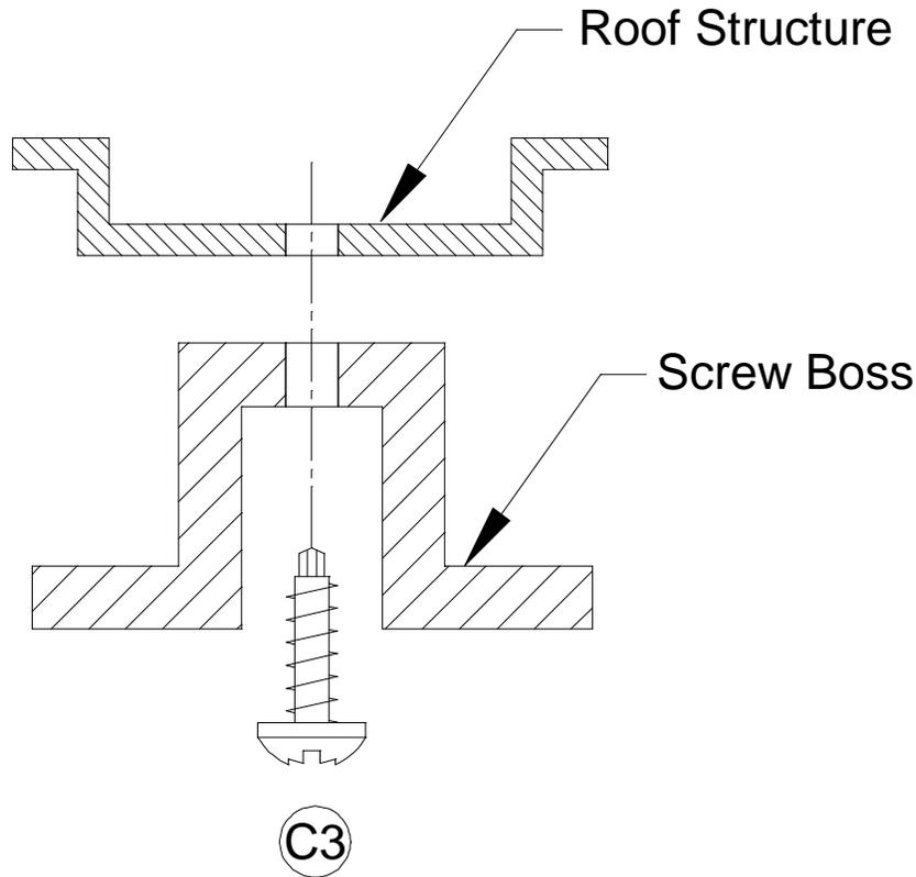
Note: If longer screws are substituted, care should be taken to prevent piercing the roof, and be sure that pan head screws and washers are used to prevent screws from pulling through the screw boss. Eight screws must be used and secured to solid structure when mounting.
