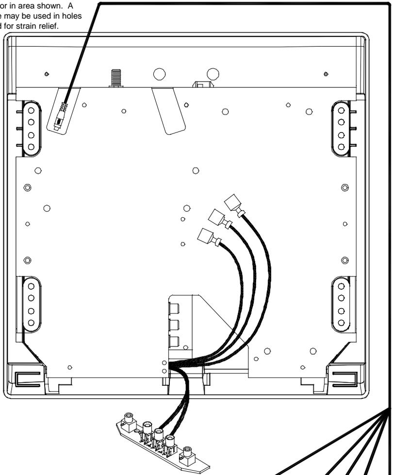
IR LED: Clean the IR window on the front of the VCP, remove the adhesive backing and apply the IR LED to IR window on the face of the VCP.
