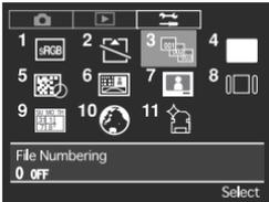
1. Press the MENU button. Press the toggle keys to select [3 File Numbering] in the setup menu and press the OK button.
