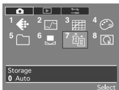
1. Press the MENU button. Press the toggle keys to select [7 Storage] in the recording menu and press the OK button.
