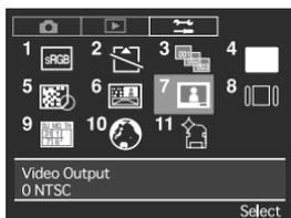
**1** Press the MENU button, and then select [7 Video Output] on the Setup Menu with the toggle key
