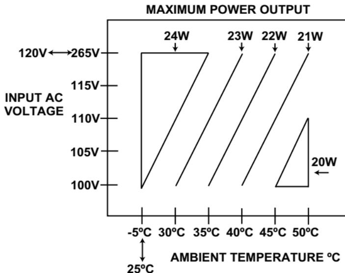
Example: If ambient is 50°C, maximum wattage is 21W max. for 120-265Vac. If unit is operated at 21W at an input voltage of 100V, the maximum ambient temperature allowed is 40°C.
