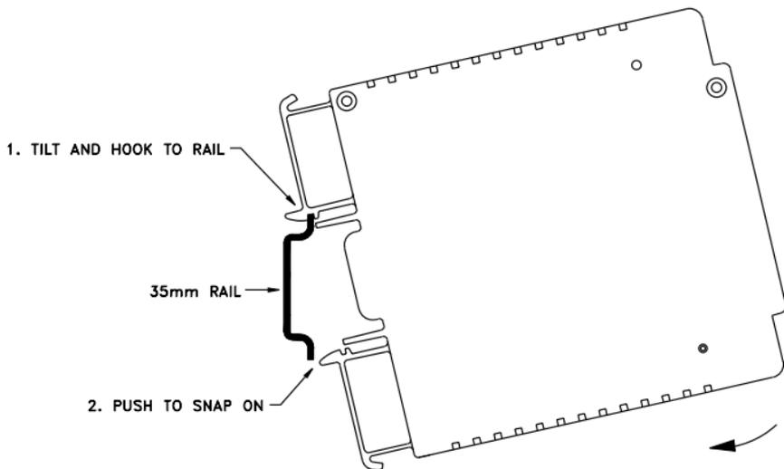
**Figure 3.2 — Mounting on 35mm DIN Rail**
