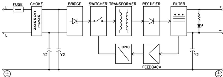
**Figure 4.1 — Block Diagram**
