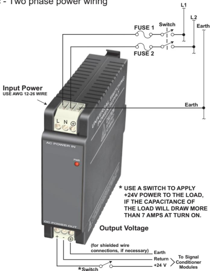
**Figure 4.3— Wiring for 230Vac - Two Phase**
