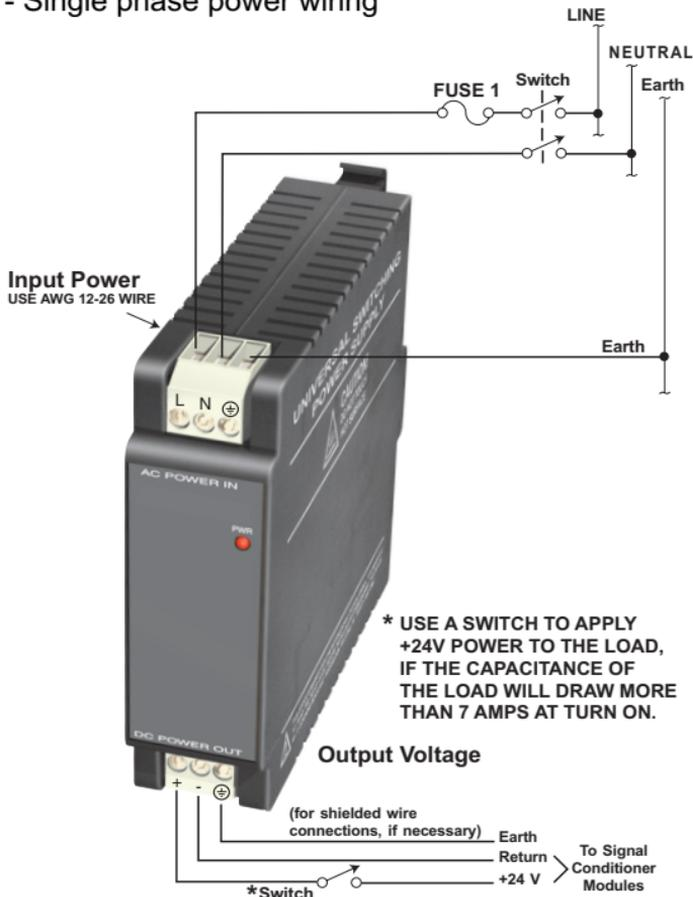
**Figure 4.2— Wiring for 115Vac - Single Phase**
