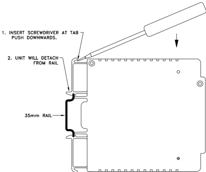
**Figure 3.3 — Removal of Unit**
