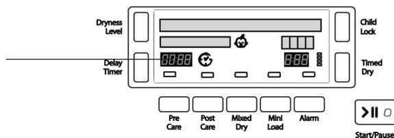
After the delay period finishes (or for all of the programme if delay not selected): The estimated Time to End of the programme for automatic programmes or the actual time remaining during the Timed programme is shown in this part of the display.
