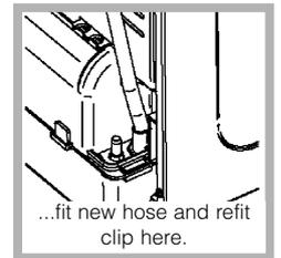
Fit a suitable length of hose to the new location shown (*see diagram*) and refit clip.
