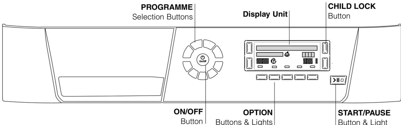
The **ON/OFF** button/light : If the dryer is running and this button is pressed, the dryer is turned off. Press again, the dryer restarts.
