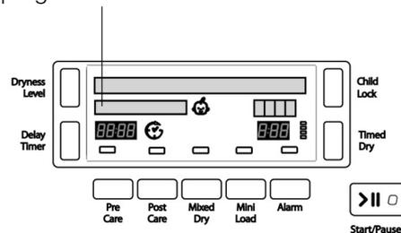
If the Mixed Dry option is available and selected this line displays when the different dryness levels have been reached:
