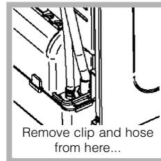
Remove the existing clip and hose from position shown (*see diagram*).
